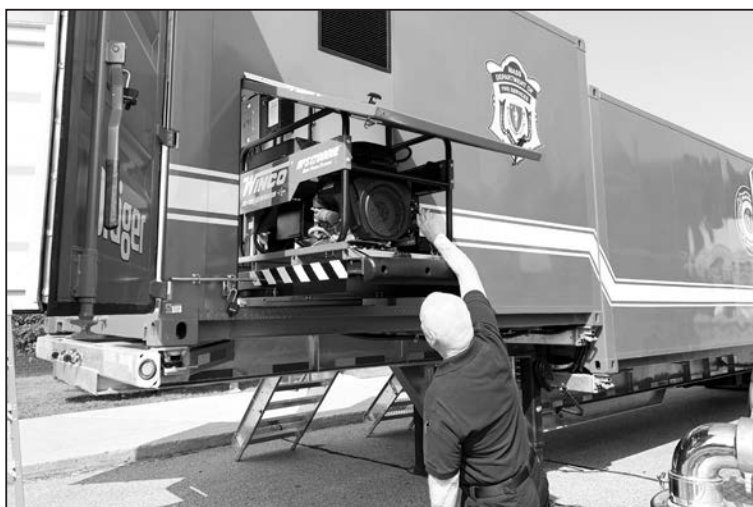
The new SCBA Maze Trailer’s modern lights, speakers, and video monitoring system are powered by an onboard generator, allowing it to be used anywhere local fire departments need it.
