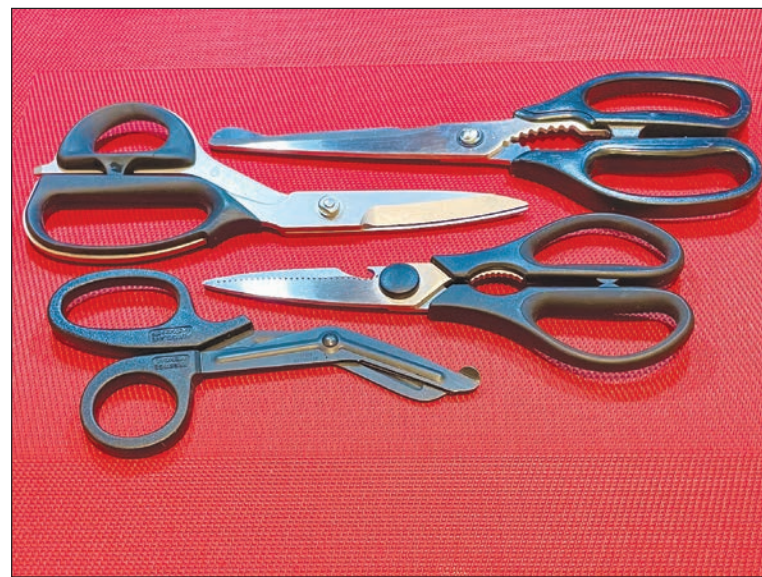
We use four types of scissors in our kitchen. Top to bottom, they are Korean scissors, heavy-duty poultry shears, utility scissors, and first-responder trauma shears.
